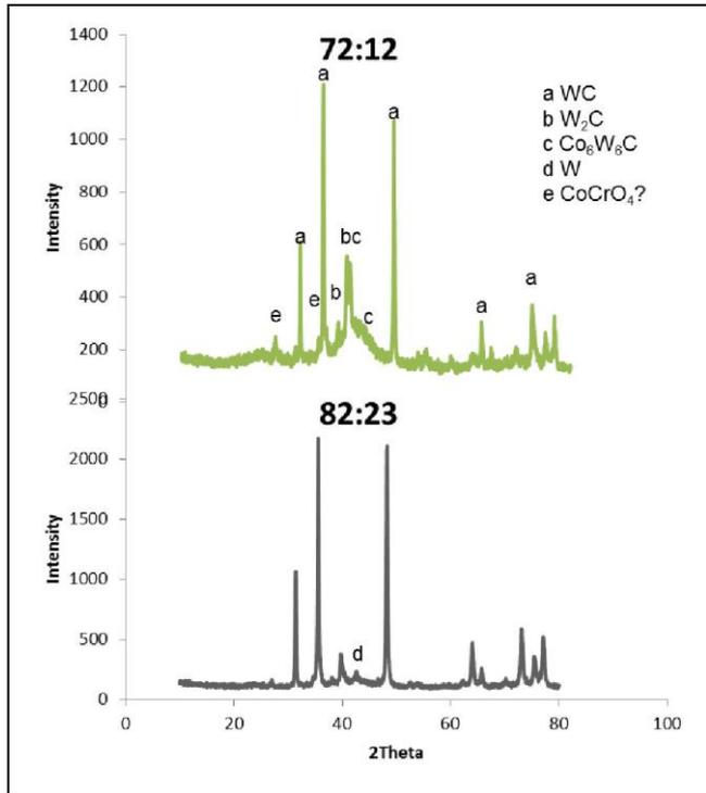
**Fig. 6.** X-Ray Diffraction Patterns, with Phases Identified for Detonation Process Conditions
