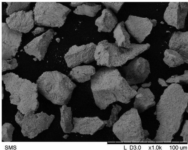
Fig. 1. WC-CoCr Cast and Crushed Powder
