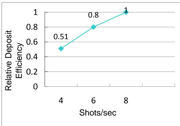
**Fig. 4.** Relative Deposit Efficiency as a function of Shot Frequency
