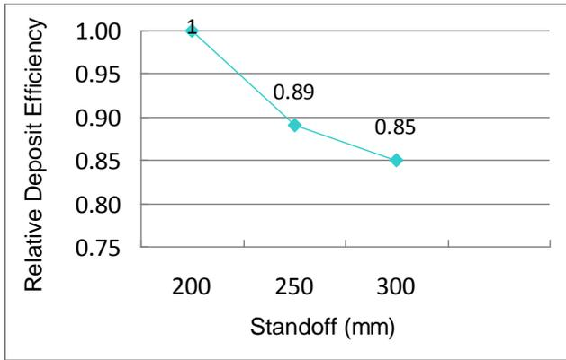
**Fig. 3.** Relative Deposit Efficiency as a function of Stand-off Distance
