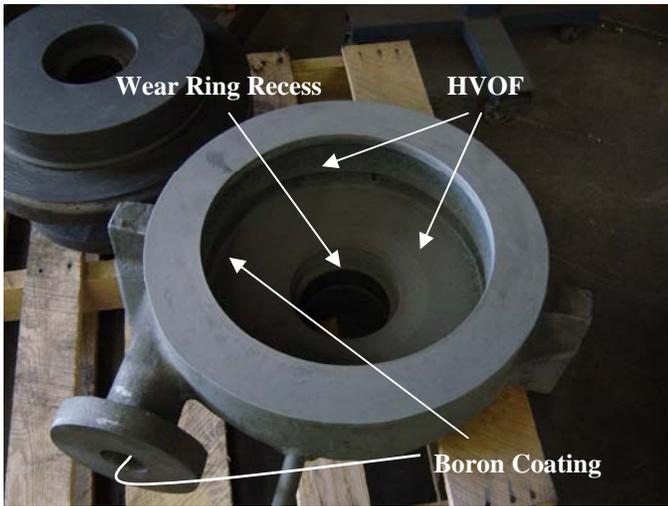
Figure 5: Centrifugal pump case showing wear ring area and coating strategy.
