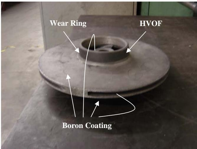
Figure 6: Centrifugal pump impeller showing wear ring area and coating strategy.
