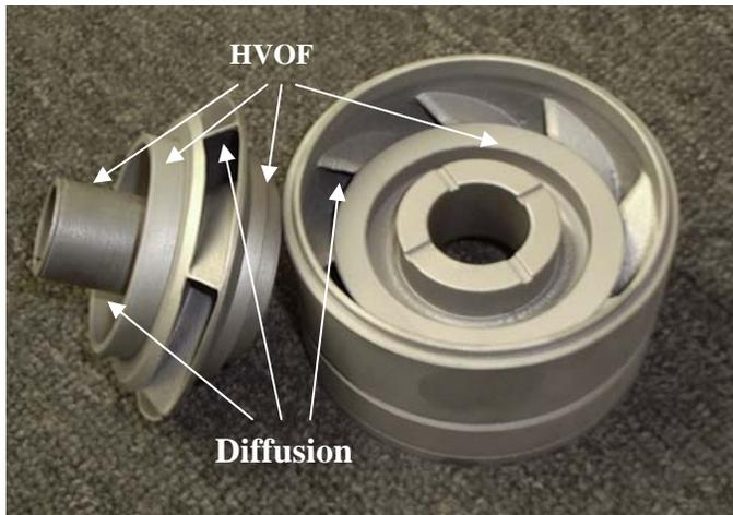
Figure 3: Example of coated impeller and diffuser showing coating strategy.
