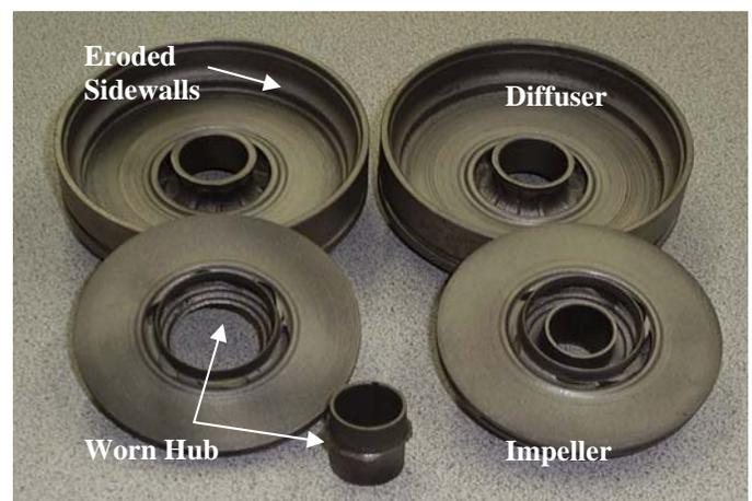
Figure 2: Worn impellers and diffusers from a multistage pump.
