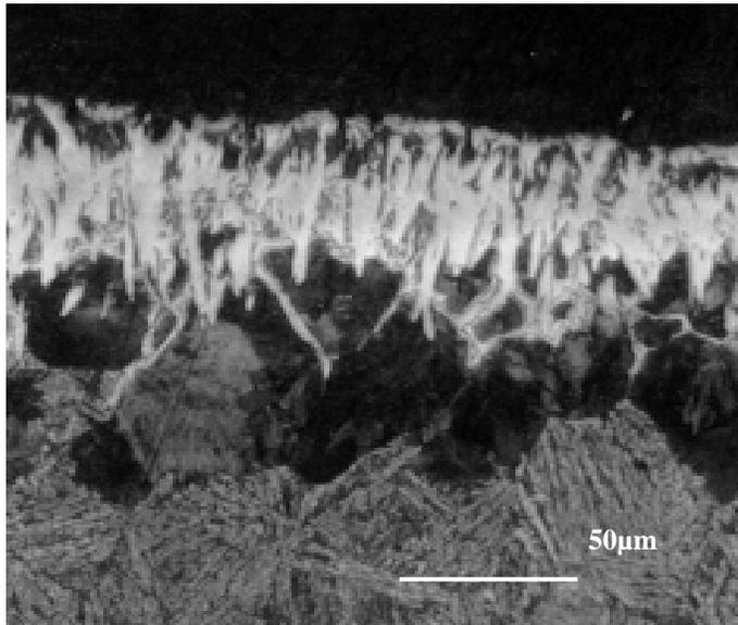
Figure 1: Boride coating on 410 stainless steel applied using pack cementation (nitric acid etch).
