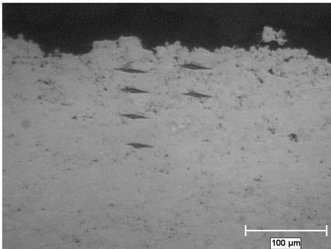
Figure 4: Cross-Section of HVOF  $Cr_3C_2-NiCr$  followed by boronized coating.
